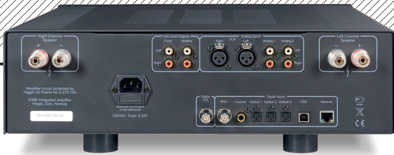
ABOVE: Substantial 4mm speaker outlets, plus fixed and variable preamp outs are joined by three line inputs (one balanced on XLR). The row of digital ins includes three optical, two coax (RCA/BNC), USB-B and an Ethernet port. A digital out (BNC) is added
